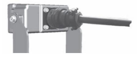
**5** Make any final adjustments to the viewing angle and tighten all bolts. The recommended camera bolt torque specification in between 17 and 20 inch pounds.
